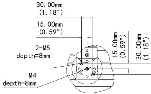
Detail A Engineering installation screw hole
